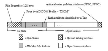
The Merge DICOM Toolkit representation for DICOM files and file meta information consists of the **MCfile** and **MCfileMetaInfo** classes, respectively.
