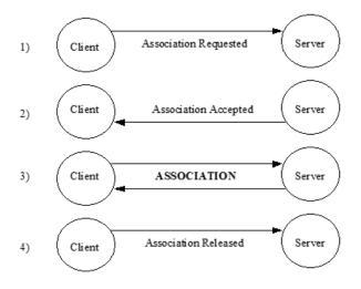
The association request proposal contains the set of services the client would like to perform and the transfer syntaxes it understands. The server then responds to the client with a subset of the services and transfer syntaxes proposed by the client. If this subset is empty, the server has rejected the association. If the subset is not empty, the server has accepted the association and the agreed upon services may be performed.
